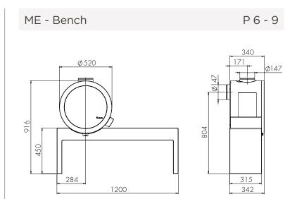
Minimum distance to combustibles:\* 100mm (rear), 700mm (side) & 700mm (above)
