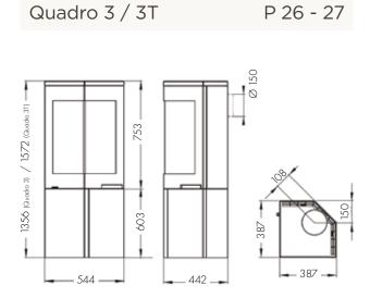
Minimum distance to combustibles:\* 150mm (rear) & 800mm (side)
