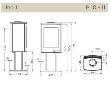
Minimum distance to combustibles:\* 150mm (rear), 500mm (side) & 600mm (above)
