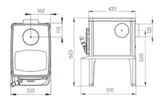
Minimum distance to combustibles:\* 600mm (rear) & 600mm (side)
