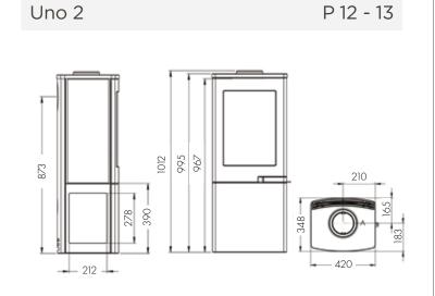
Minimum distance to combustibles:\* 150mm (rear), 500mm (side) & 600mm (above)
